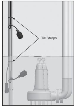
Functionally test the level measurement and ensure proper operation of the system by filling the tank.
