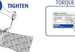
Tighten the Grip's bolts to the right torque shown on the product label. When you finish, re-check the torque again.
