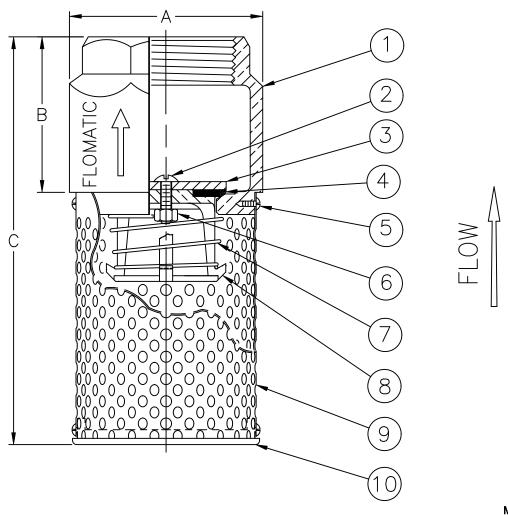
Open Area: 35-50% Max Temp 180°F (82°C) Max Pressure 250psi (18bar)
