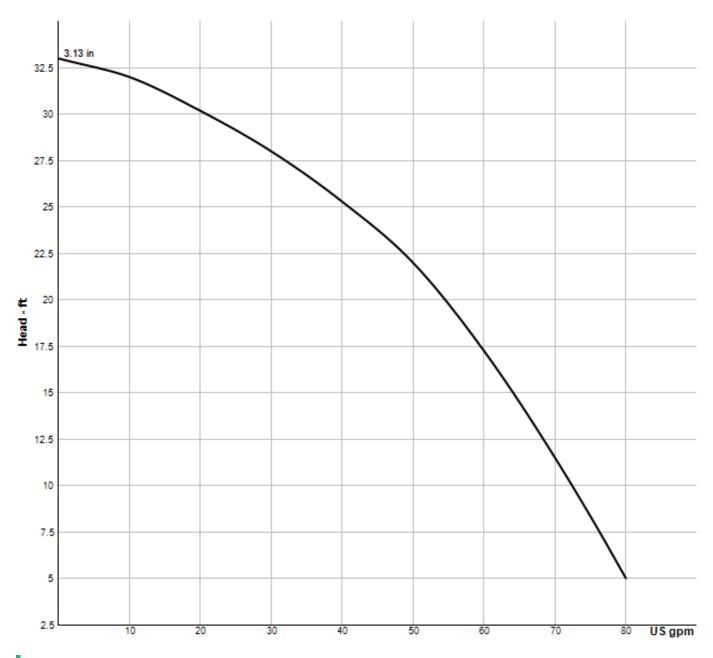
Testing is performed with water specific gravity of 1.0 @ 68°F (20°C), other fluids may vary performance
