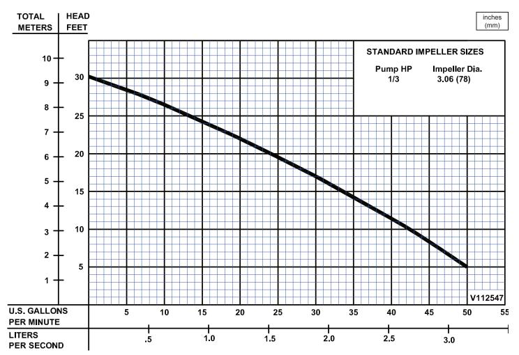
Testing is performed with water, specific gravity 1.0 @ 68° F @ (20°C), other fluids may vary performance
