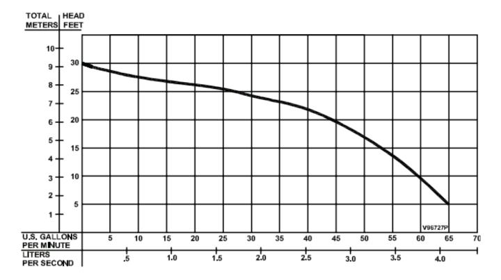
Testing is performed with water specific gravity of 1.0 @ 68°F (20°C), other fluids may vary performance
