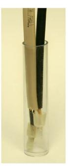
Pull splice out of vial and mix epoxy throughly. Pour epoly into vial to about 2/3 full. Shove spliced wires down into epoxy until seated at bottom of vial. Store upright until epoxy hardens.
