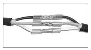
c. To shrink the insulated heat shrink tubing, apply moderate heat with a propane torch or heat gun (or any tool that will provide adequate heat.) Caution: Keep the torch moving; too much concentrated heat will damage the tubing.
