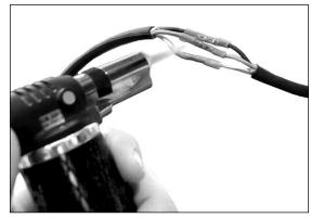
d. When tubing begins to shrink, increase concentration of heat at the edge of the butt connector. As the tube collapses on the wire, work heat out to each end until entire tube has collapsed tightly around the wire. Enough heat should be applied to melt the sealing glue on the inside of the shrink tube. As the tube collapses around the wire, some sealant should ooze out of the end of the tube providing a water tight seal.
