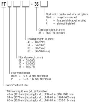
66-in. (1676-mm) housing for MLL of 85-112 in. (2159-2845 mm)
