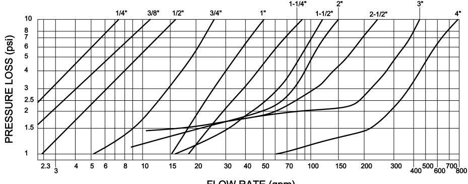
FLOW RATE (gpm) verified by independent lab
