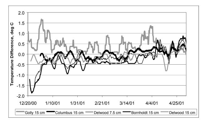
Figure 7. Temperature Difference Between the Emitter Line and the Soil Between the Emitter Lines. (Negative numbers indicate the emitter line is colder than the soil between emitter lines. Data presented is a running 3-day average of logged temperature readings).
