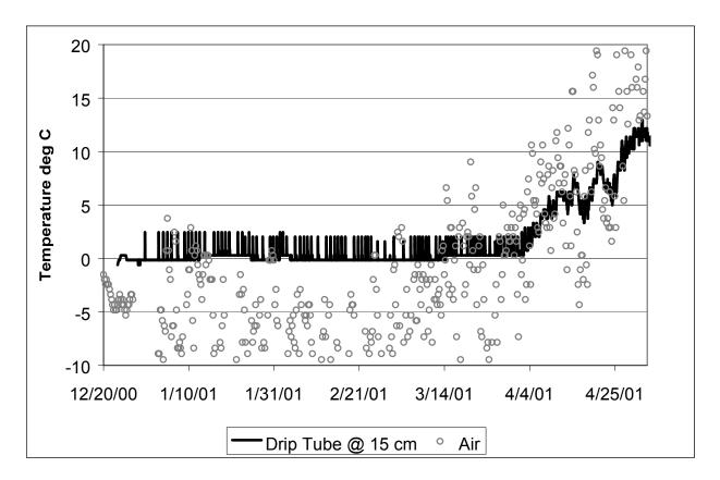
Figure 4. Columbus Elementary School. Temperature of the Emitter lines with 15 cm of Soil Cover.
