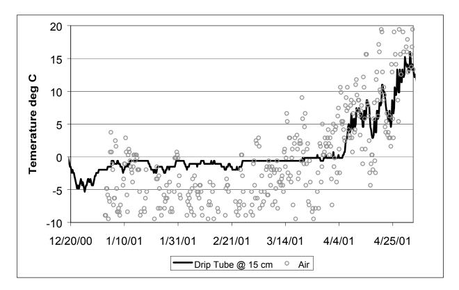
Figure 3. Bornholdt Residence. Temperature at the Emitter Lines with 15 cm of Soil Cover.
