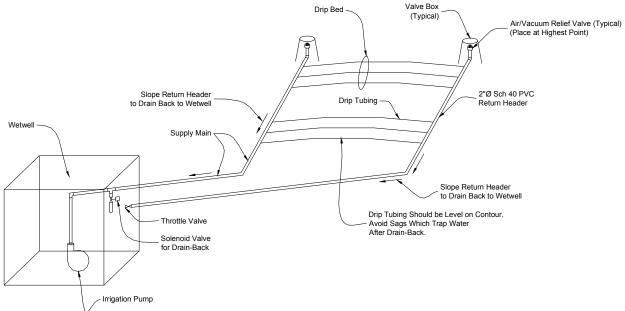
Figure 1. NAWE Cold-Climate Drip System Schematic.
