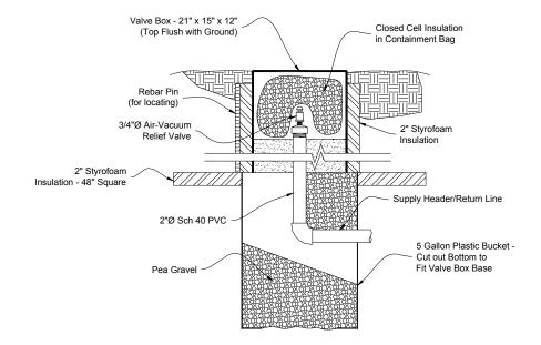
Figure 8. Recommended Air/Vacuum Relief Valve Box Insulation Method.
