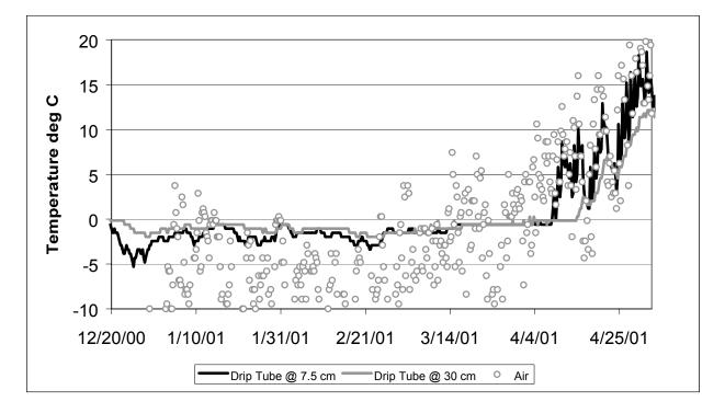
Figure 2. The Greens of Dellwood. Temperature of the Emitter Lines with 7.5 cm and 30 cm of Peat Cover.
