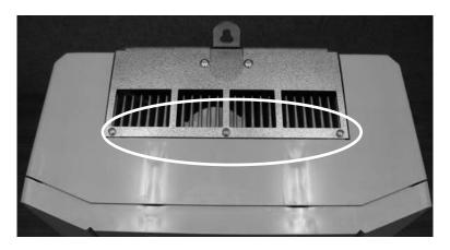
2. Remove the screws using a Philips screwdriver. DO NOT discard these screws as they are used to install the heatsink cover.
