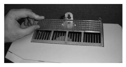
4. Pivot the heatsink cover to lay flat against the topside of the mounting bracket of the drive. Make sure that the retention hooks are properly positioned to grasp the sheet metal.
