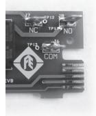
Either or both sets of contacts can be utilized to reflect drive status.
